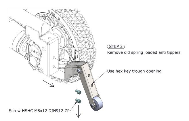
For mounting new spring loaded anti tippers follow the steps in reverse.
